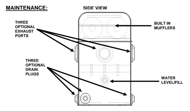
Maintenance must be performed periodically so that sludge does not build up in the bottom of the enclosure. To clean the water chamber, drain the water by removing one or more of the three (3) pipe plugs located at the bottom side of the enclosure. Remove the ½ inch pipe plug on the opposite end of enclosure approximately 5½ inches from bottom of enclosure, flush water chamber with clean water until the water exiting is clean.
