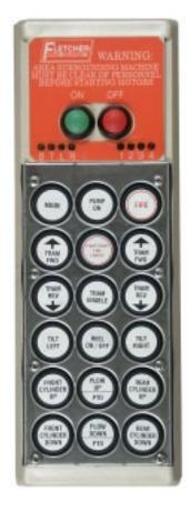
mobile roof support systems (MRS). Due to the location in which these machines operate – under unstable and caving roof conditions, there is no safe means of operation other than by remote control.
